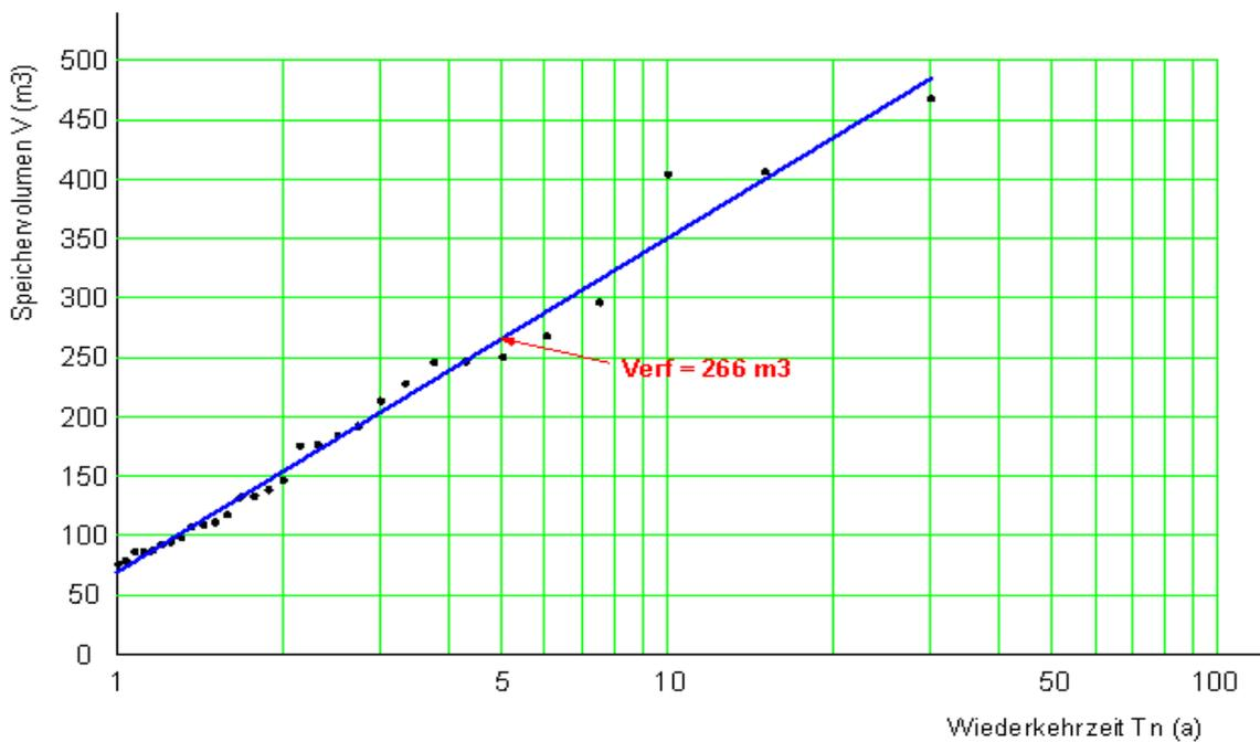
$V = 281,301 * \text{Log}(Tn) + 68,999; \quad Tn = 5,0 \text{ a}; \text{ Verf} = 266 \text{ m}^3$
